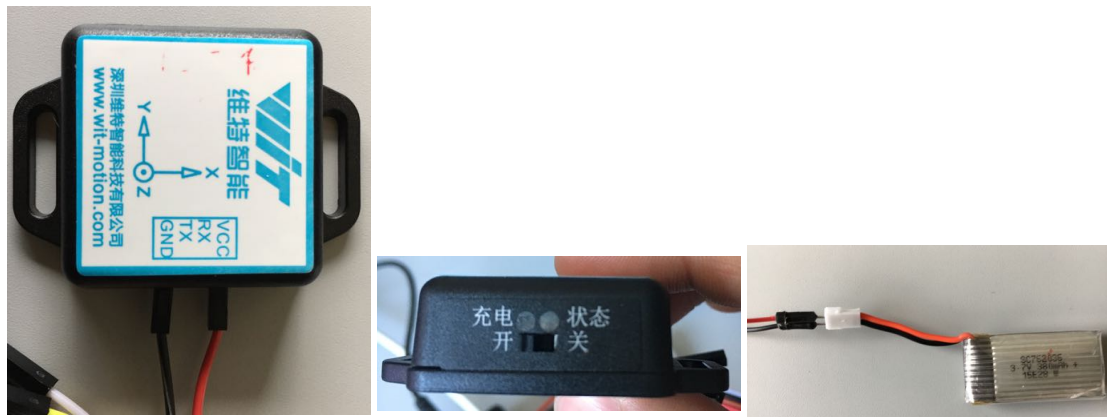
Figure 1: Bluetooth JY61 MPU6050 module and battery
